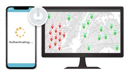
This log can then be used to feed a visual map based web application, with the passed or failed attempts being illustrated by location markers. A concentration of failed attempts within a specific area on the map could indicate a possible counterfeiting source.
